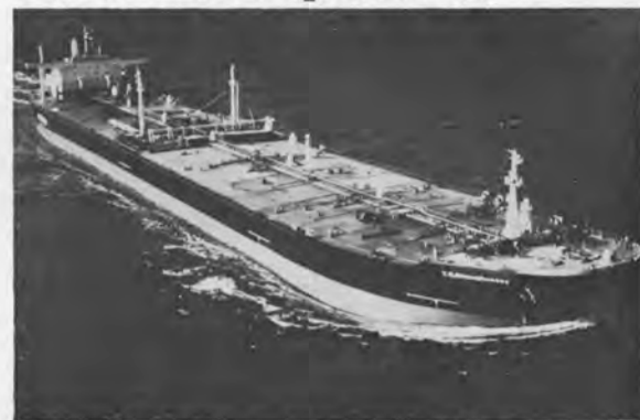
The T.G. Shaughnessy, 1,109 feet by 170 feet by 87.6 feet, will be chartered to Gulf Oil Corporation.
