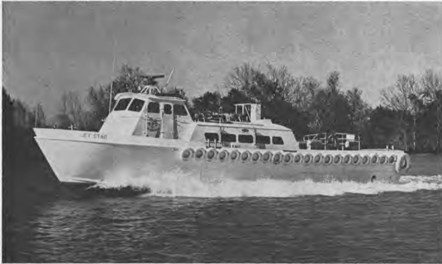
Powered by a pair of turbine engines, the 65-foot crew boat Jet Star will be used to transport crewmen to offshore oil wells in the Gulf of Mexico.
