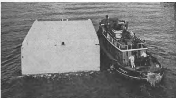
McAllister Brothers Inc. tug Eileen McAllister shifts LASH lighter at terminal operated by Universal Terminal and Stevedoring Corporation. The tug, originally designed for service on the Erie Barge Canal, has a low silhouette that enables it to work under the cantilever extensions at ship's stern.
