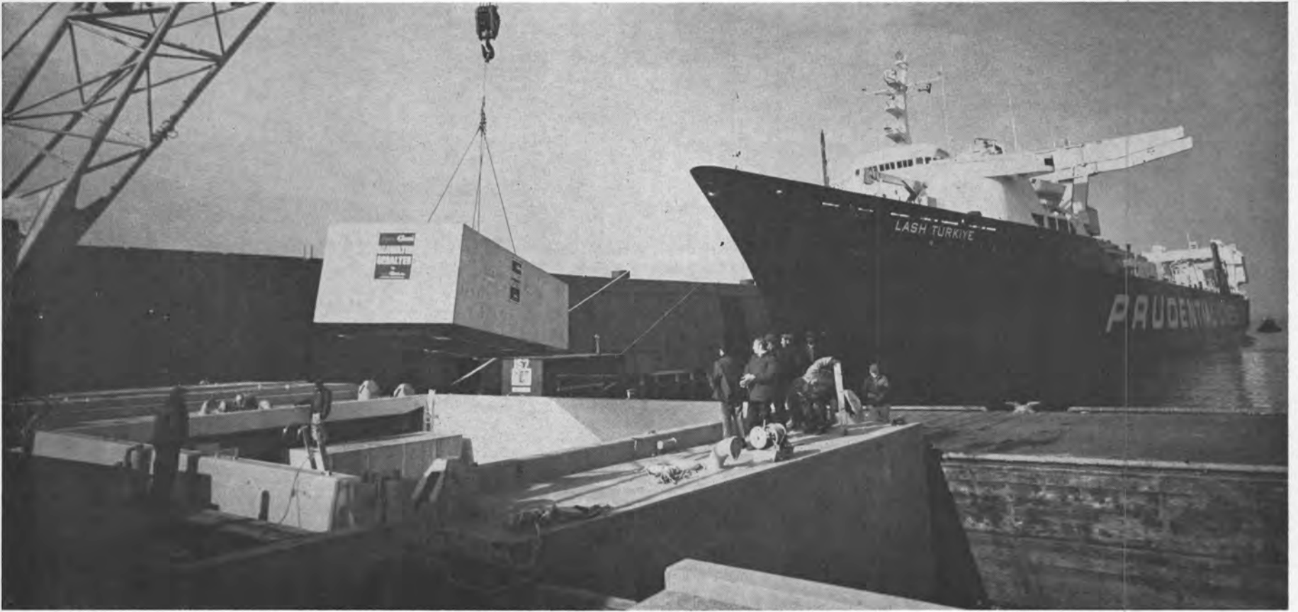
Longshoremen at Bush Terminal, Brooklyn, N.Y., unloading cargo from a lighter that was delivered by the LASH Turkiye.
