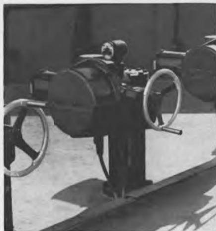
This operator controls a tank valve deep in the hull.
