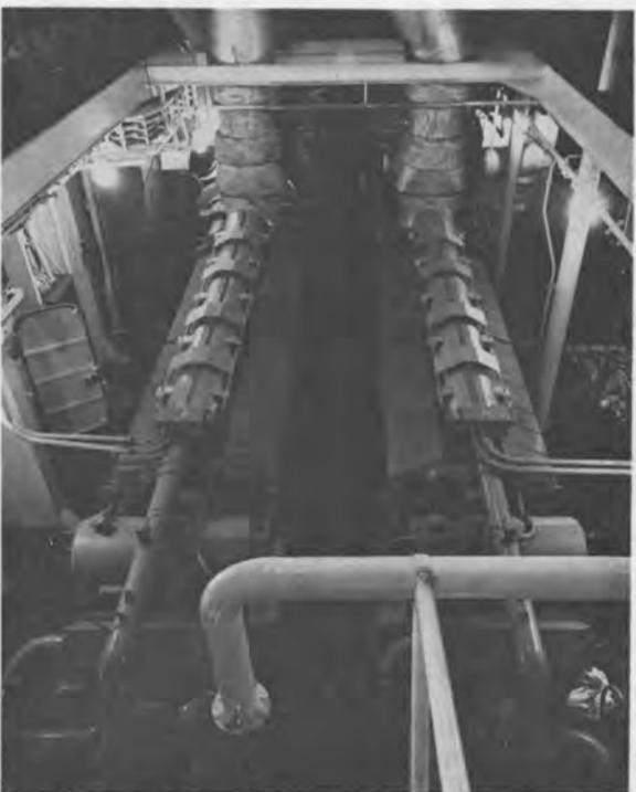
Starboard engine room showing two 3,500-hp General Motors Electro-Motive diesel engines.
