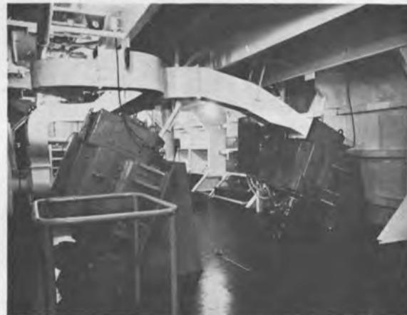
Aft thruster motors with vent ducts looking to starboard.
