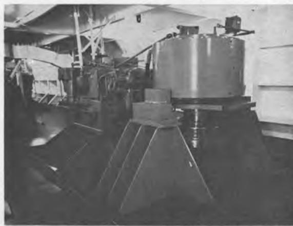
Port rotary actuator steering gear.
