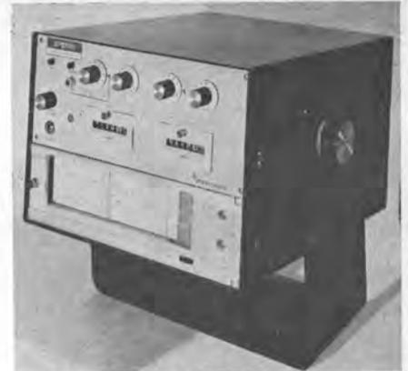
With the SR-500 Omega receiver a navigator can fix his position within minutes.
