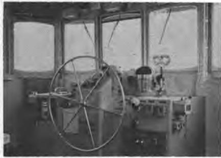
Pilothouse of the YTB-803 class tugs features a control console containing all maneuvering control and navigation components. The PSI electric steering control stand with 40-inch wheel is located at the center of the console. Auxiliary non-follow-up steering control levers are mounted at each side of the console.
