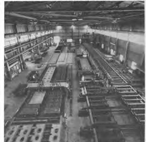
The fabrication building at Litton's Erie plant. Panels of 48-foot-long by 90-inch-wide plate with three stiffeners are produced on a production line in this building.
