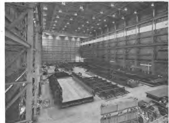
The 48-foot plates are moved to the assembly building via special trailers. The period from reclaiming steel from the storage yard to the module rotation is about two weeks.
