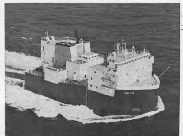
STUBBY, comprised of only bow and stern welded together, is shown leaving its birthplace at Litton's Ingalls Nuclear Shipbuilding yard in Pascagoula, Miss., to steam 2600 miles to Lake Erie, where the modular midbody was inserted to become the largest ore carrier on the lakes.
