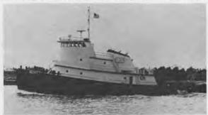
Profile view of the new 120-foot ocean tug Betty, built by Halter Marine Services, Inc., New Orleans, for Southeastern Drilling Company, Houston. Betty is the first in a new series of tugs designed and built by Halter. The tug is powered by two 16-cylinder GM EMD 645E2 diesels that develop a total of 4,200 horsepower. The Betty will be used by Sedco for towing pipelaying and derrick barges.
