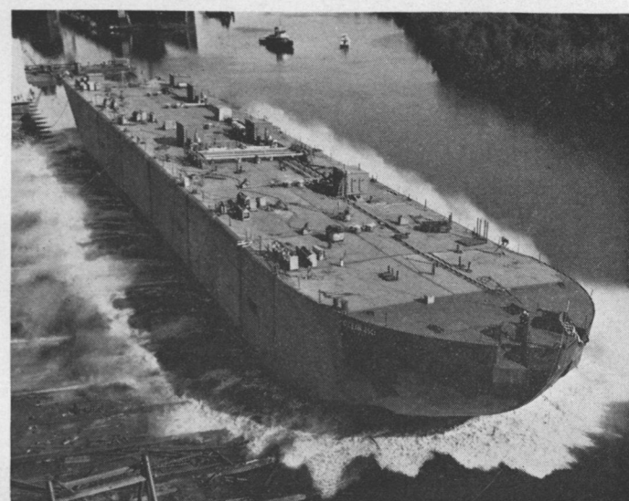
SEAGOING TANK BARGE 546 x 85 x 40 ft Capacity: 30,000 bbl
