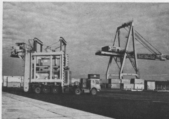
A six-wheel, triple stacking straddle carrier unloads a 20-foot container from a CP Express trailer truck at CP Ships' new container terminal at Quebec City. In the background is the terminal's $900,000 Portainer crane.
