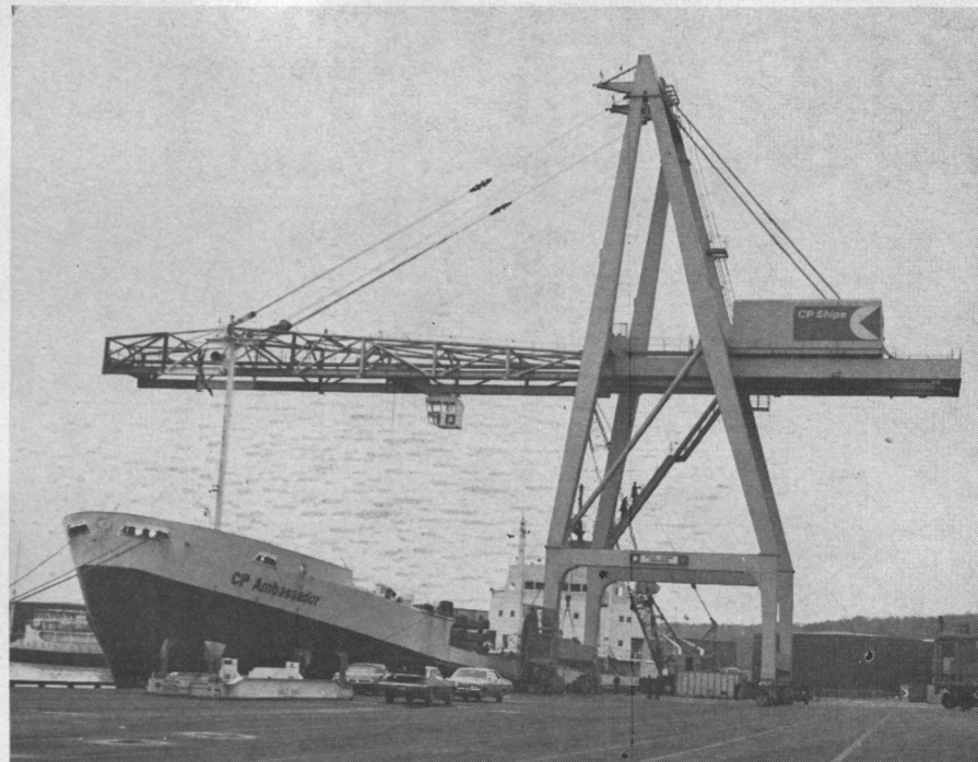
CP Ships' vessel Beaverack was stretched to increase its capacity to 322 containers and renamed the CP Ambassador. The $900,000 PACECO-Vickers Portainer Crane at CP Ships' new highly mechanized container terminal unloads the CP Ambassador at a rate of almost 40 containers per hour. The new facilities permit this vessel to completely unload and reload in 30 hours. The terminal, which has a weekly throughput of 1,600 containers each way, is the key to CP Ships' successful North Atlantic container services.
