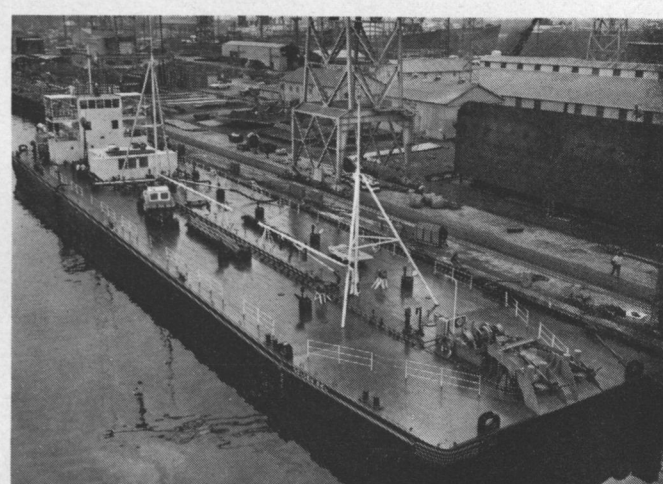
SELF-PROPELLED BUNKERING BARGE 260 x 55 x 17 ft Capacity: 255,000 bbl
