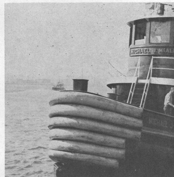
The new type non-marking Uniroyal fender is shown on the Michael J. McAllister now operating out of Norfolk, Va.
