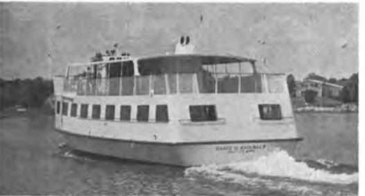
85' PASSENGER FERRY: Built for fast and rugged service in the Straits of Mackinac on Lake Huron between Mackinaw City and the very popular resort island of the same name. She is certified for 450 passengers and joins a second Blount ferry on the same run.
