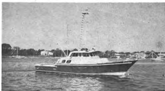
57' 500 H.P. TEST BED: Built and operated by Blount for research and development of power pods, sound attenuation and new offshore fishing methods. The propeller shaft and tailshaft bearing of this vessel can be removed and replaced without drydocking.
