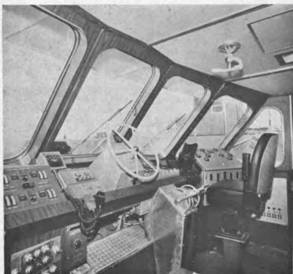
All controls for operating the Avalon are centered in the pilothouse in full view of the helmsman and deck officer.
