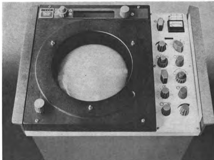
Indicator Unit of New Decca radars — with 9" dia. Scope and nine range scales — 1/4 m to 48m.
