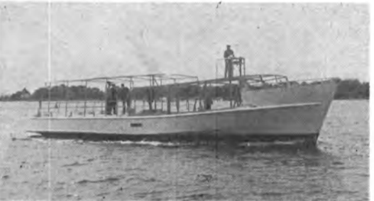
65' SIGHTSEEING HULL: This 200 passenger hull was built as a "hull with engines only." The owner will finish the superstructure. She will operate out of Bar Harbor, Maine for sightseeing in the Acadia National Park.
