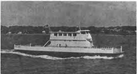
100' DOUBLE END TWIN SCREW FERRY: Delivered via the Erie Canal, this vessel joined two Blount sister ferries on a famous Lake Erie run between Sandusky and Kelley's Island. Powered by two 350 H.P. diesels, she makes 13 knots and carries 15 cars.
