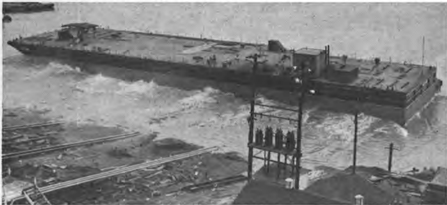
Built for Houston Contracting Company, the new barge measuring 370 feet by 85 feet by 24 feet was designed to lay oil and natural gas pipelines in any seas of the world.
