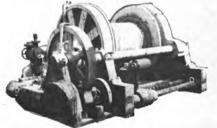
Single drum, capacity 2000' of 2" wire rope, cylinder size 9" bore by 10" stroke.
