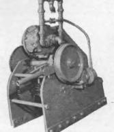
For Barge & General Marine Use Winch duty 11,000 lbs. @ 39 FPM. Drum capacity 115 ft. of 1" wire. Drum size—11". Air motor mfg by Gardner-Denver—type MKB-A—reversible —11.5 HP @ 100 lbs. pressure. 1" Pipe connections for air. Typical serial No. 458307. Just removed from unmanned barge. Good operating condition. 7 Units, with motors, available.
