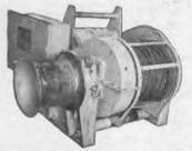
24 - American Hoist & Derrick Company Cargo Winches, 12-R.H., 12-L.H., single drum, single gypsy, Mfgs. No. 67696, rated 7400 lb. line pull at 220 FPM, total stowage capacity 709' of 78" wire rope, powered with Westinghouse Motors, 50 HP, 230 volts DC, 600 RPM, compound wound, Type CK, Frame 9, complete with Control Panel, Resistors and Master Switch. All units are of Recent Manufacture.
