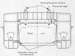
Figure 5—Section through straddler barge carrier.
