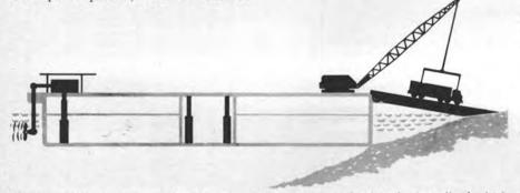
The special barges have their own powerplant, crane and landing bridge all of which stow within the barge when not in use.
