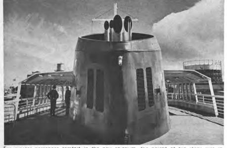
For greater passenger comfort in the new solarium, the neight of the stack was increased by three feet. The solarium is heated electrically.
