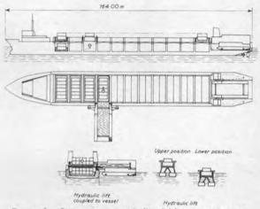
Figure 3—Barge carrier with floodable compartments.
