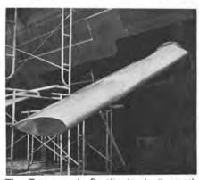
The Tustumena's Pacitic Mark X stabilizers are of the horizontal, swing-out oscillating fin type.
