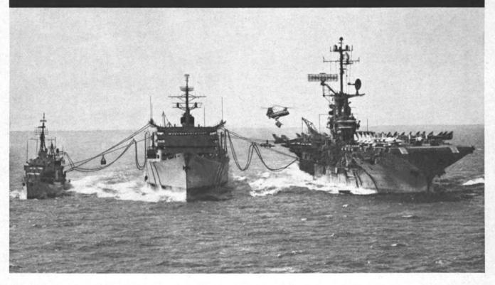
The U.S. Navy tackled a problem: how to transfer at sea the high volume of cargo needed for effective fleet operation. Through competitive bidding, Western Gear obtained contracts to turn a concept into working hardware. The resulting replenishment-atsea system is unique in its function, and is a model of effective design and rugged construction. It meets the Navy requirement
