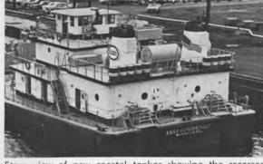
Stern view of new coastal tanker showing the recessed outboard propulsion drive units.
