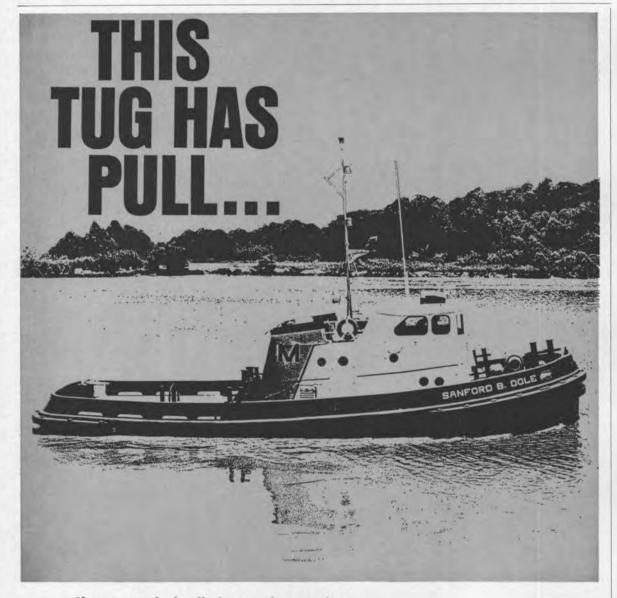
If ever a tug had pull, this one does. Made to take it, powered by two 500 HP Diesel Engines, this tug was delivered to Hawaii to maneuver ocean liners for Matson Navigation. Every piece of her was made to last. 65' x 20' x 10'6" and every inch a champion. Call on the master builders at ZIGLER SHIPYARDS to supply you with a tug that has pull. They never fail. Ask Zigler to send you a brochure.
