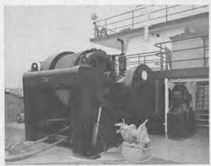
The 300,000 pound single-line-pull waterfall-type double-drum winch built by The Red Fox Machine & Supply Co., aboard the Penrod Drilling Co. owned Hippo.
