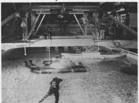
Much of the entire facility's key operating equipment is on a traveling bridge across the wave tank at Chicago Bridge & Iron Company's Marine Research Center. Shown here is the testing of an offshore storage and tanker loading facility, with divers viewing the wave actions.
