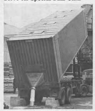
International Ferry Freight Ltd. (I.F.F.) of England has developed in conjunction with I.C.I. plastics division a system for carrying granular chemicals in bulk in standard ISO box containers, which are back-loaded with general freight, thereby eliminating the costly return of empty containers. The containers and tipping skeletal trailers used in the system are being manufactured and marketed by York Trailer Company Ltd., Corby, Northants.
