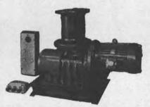
MOTOR: 10 HP—totally enclosed—fan cooled continuous duty — horizontal flange mounted — special shaft & oil seal fitted—440/3/60—1760 RPM. CONTROL: Marine type water-tight pushbutton—forward/reverse/stop—watertight starter
