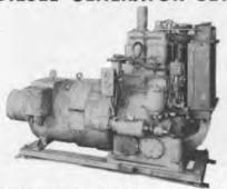
2 Available. 30 HP Nordberg 2-cylinder diesel engine — 4½" bore — 5½" stroke — 4-cycle—1800 RPM—167 cu. inch displacement. Electric starting. GENERATOR: Kato Engineering Co.—20 KW A.C.—1800 RPM—120/240 volts DC—D.C. exciter. Panel boards have Regohm voltage regulator. lator. Panel is rigged for automatic standby control.
