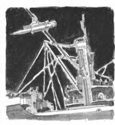
Fast Automatic Shuttle Transfer (FAST) is a system we built for the Navy. It transfers missiles between ships at speeds up to 900 feet per minute—yet lets them arrive with less than 2 G's shock!
