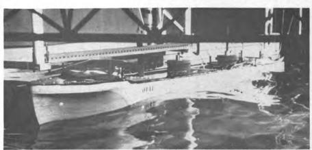
Model of barge undergoing tests in model basin. Ship-form bow proved to be best.
