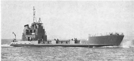
Operating out of Seattle on a 2,700 mile run to Alaska and the Aleutians, the Skilak, first of the Super-U vessels, carries freight and oil, lighters from ships offshore to the rugged beaches, and tows barges. She runs light at 8 knots, and has towed 1,000 ton barges at 6 knots (Below) The U. S. Navy has purchased 12 similar crafts in a military version.
