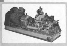
WESTINGHOUSE Turbines, 440 PSI, 740° F, with Westinghouse Generators, 250 KW, 120/240 DC.
