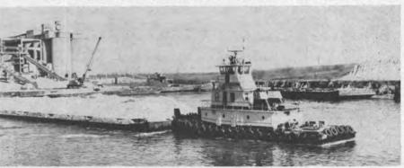
The entire power requirements for the Robin Rose were designed and supplied by Stewart Stevenson. The boat can push three 200-foot light barges at  $10\frac{1}{2}$  miles per hour and 8 miles per hour loaded.
