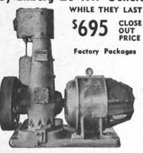
120 volts DC-400 RPM-drip-proof marine type. 2-Wire direct connected set. Reciprocating 6 type E vertical self-oiling steam enginepiston valve-220 lbs PSI-80 lbs. BP.
