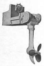
Model 0-7 unit in stock. Powered by twin GM 8 lowered mechanically. 7' from bottom of unit to propeller hub center. Weight about 20,000 lbs. Propeller speed 308 RPM. Unit can develop up to 500 HP. Formerly used on Cargill Grain Co. barge "Carpolis". Actual photo on request. Can be demonstrated running in shop.
