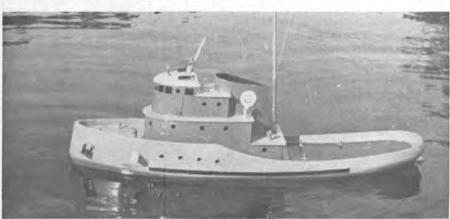
Model of tug with hydraulically operated connection extended just forward of house.
