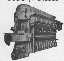
(4)—10 Cylinder—2-cycle—1800 HP @ 800 RPM. 8½x10—air starting—reversible. Complete with Harrison coolers, sylphon valves, strainers, filters, etc. For immediate delivery.
