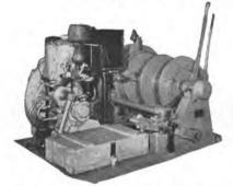
Small general purpose winches, mfg by Jaeger. Rated 2500 lbs @ 75 FPM. Driven by air-cooled Enfield single Cylinder diesel engine. Declutchable free spooling drum has center flange which can be removed if required. Excellent for small vessel use and general purpose service on all vessels. Has spare parts box. Weight about 1500 lbs.
