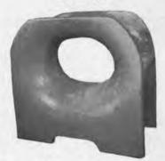
Clear opening 10" x 14" - 7" radius - with extended legs for welding to deck. Use as double or single bow chock. OAL 28" on base - OAW 14" - OAH 2734" - Cast Steel.
