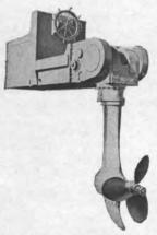
1 Model 0-7 unit in stock. Powered by twin GM 6-71 diesels with hydraulic clutch & electric steering. Propeller diam. 64" pitch 48". Tailfin raised & lowered mechanically. 7' from bottom of unit to propeller hub center. Weight about 20,000 lbs. Propeller speed 308 RPM. Unit can develop up to 500 HP. Formerly used on Cargill Grain Co. barge "Carpolis". Actual photo on request. Can be demonstrated running in shop.
