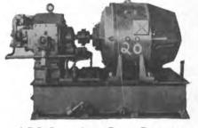
**AP3 Steering Gear Pumps** Northern Hydraulic (variable stroke) and Hele-Shaw Hy-\$1750 draulic.
