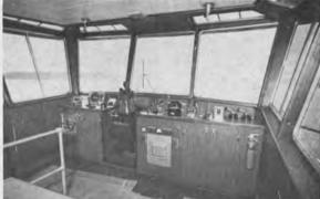
Pilothouse features overhead windows for view of ships when performing docking operations,
