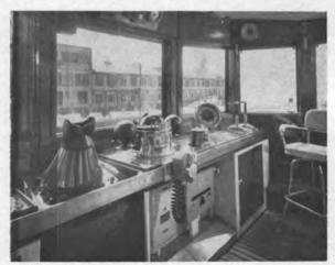
Wheelhouse has equipment conveniently located for easy use by the tua's master.
