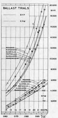
Figure 4-Ballast trial results for six ships.
