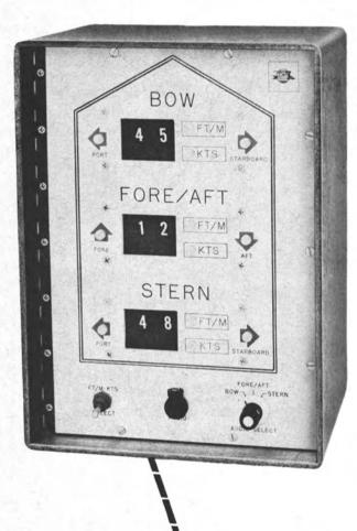
A precision docking sonar system which utilizes the Doppler principle to provide absolute "overthe-bottom" velocity information for berthing of super vessels.
