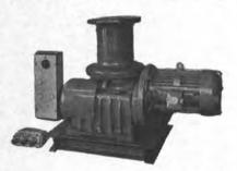
MOTOR: 10 HP—totally enclosed—fan cooled—continuous duty—horizontal flange mounted—special shaft & oil seal fitted—440/3/60—1760 RPM. CONTROL: Marine type water-tight pushbutton—forward/reverse/stop—watertight starter-box—rated for 40 sterts per hour—triple pole contactor with silver contacts, thermal overload relay end trip adjustment. DIMENSIONS: Barrel 10" diameter—Flange 10" diameter—approx. 26" wide and 36" long.
