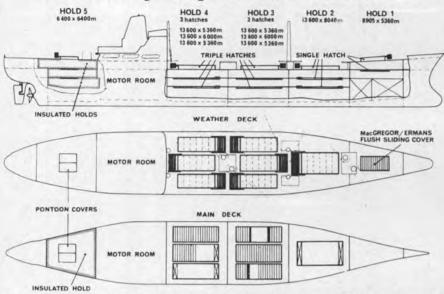
Profile and deck plans of 12,000-dwt cargo ships to be built in Brazil and equipped with MacGregor hatch covers. A total of 24 of these ships are to be built.
