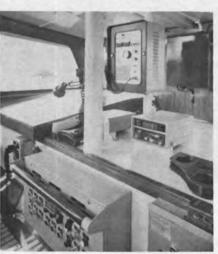
Radio equipment and automation panel is located on aft bulkhead of wheelhouse.
