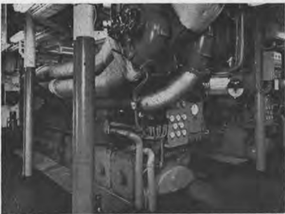
Deutz Diesel main engines provide twin-screw propulsion.
