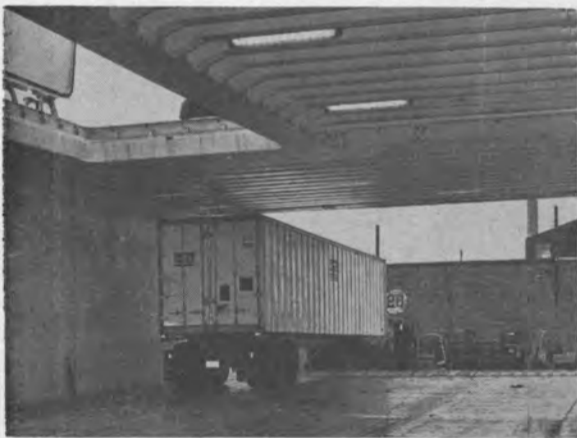
Trailer being backed onto the main deck over stern ramp.
