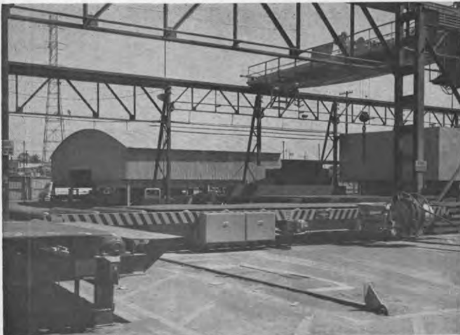
Figure 1—Cleaned and painted steel is transferred to next operation by transfer car shown above. The material goes either to burning operations or to Collocator.
