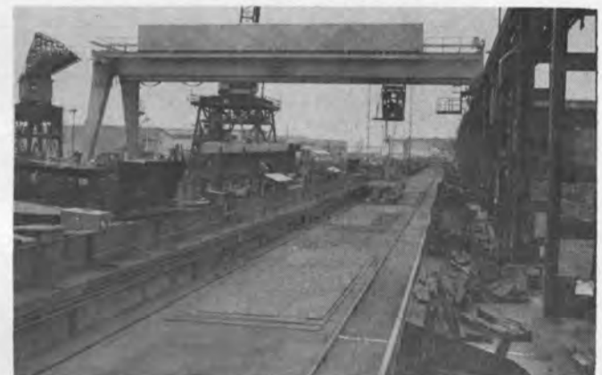
Figure 9—Crane lifts plate from between Collocator track and moves it to proper subassembly platen. Whirley crane transfers completed assembly to transporter for building ways.
