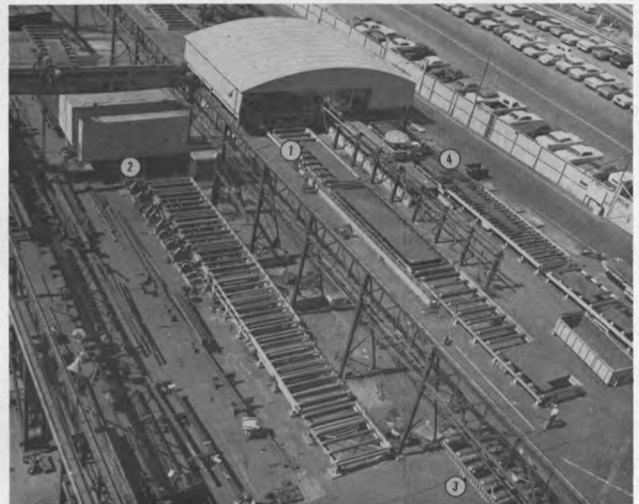
Figure 6—Overall view of Sections 4-7 (taken prior to completion) shows arrangement of flame planer (1), beam welder (2), transfer car (3), and profile cutting (4).
