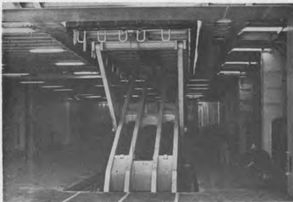
Elevator is raised to weather deck by operator at right.
