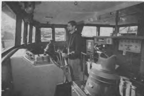
Island King's wheelhouse, fitted with latest in navigational and control instrumentation, including automatic pilot.
