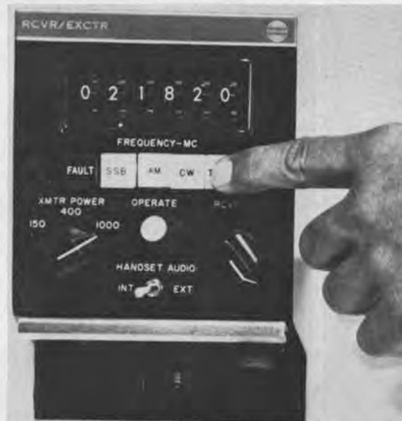
The automatic tuning device from Collins' MR-102 HF/SSB Maritime System. All stages, including the antenna, are automatically tuned for maximum efficiency by setting up the proper frequency and pressing the tune button.
