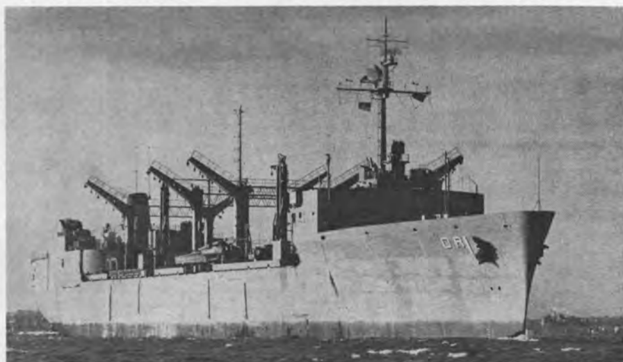
NAVY'S NEWEST—First of a new class of U.S. Navy supply ships, the USS Wichita (AOR-1) heads to sea from the Quincy, Mass., shipyard of General Dynamics for her maiden trials. The 659-foot-long vessel, displacing 37,360 tons when fully loaded, is designed to replenish operating forces at sea with petroleum products, refrigerated and dry provisions, consumables and ammunition, including missiles. Named after Wichita, Kansas, the ship was launched March 16, 1968. She is the first of six ships of her class to be built by the Quincy division of General Dynamics.
