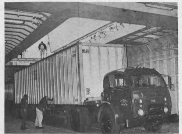
Trailer is unhitched from tractor on the elevator platform.
