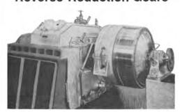
1-starboard, ratio 2.292:1, rated 2000 HP, with Fawick Clutches.
