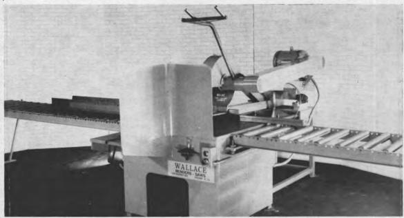
Conveyor feed and discharge units shown to the right and left of this 20" 2600 series shown are optional extras. This is an ideal set-up for the modern "Service Center" or Structural Shop.
