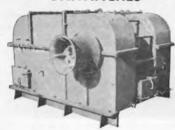
LAKESHORE UNIWINCHES, with Allis-Chalmers Motors, 50 HP, 230 Volts DC, complete with
