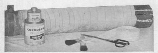
This deck steam pipe was repaired by CORDOBOND method. After one year the pipe was renewed as it fractured beyond repaired part, and the repaired part was still sound for pressure service.
