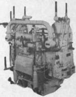
7½ C.F.H. at 3000 P.S.I.—vertical 3-stage—600 RPM. Motor 22.5 HP—440/3/60—600 RPM—drip-proof self-ventilated—squir-rel cage—ambient temp. 50°C. Good
