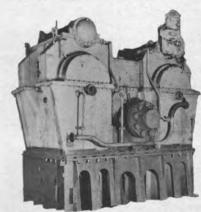
AP2 VICTORY SHIP REDUCTION GEAR Westinghouse 6000 HP double reduction gear. RPM: HP pinion 5410—LP pinion 3907. Propeller output 100 RPM. Serial A-1620. Location Baltimore.
