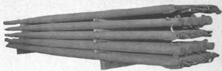
Liberty type—5-ton cap'ty—tubular taper—55'4" long. Center O.D. 15.3"—O.D. ends 8" to 8.6"—standard fittings \$465.00 EA. Victory type steel cargo booms-5-ton-48'9"-tubular taper-VC2-AP2 type .....
