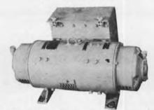
Type CHT-211761. INPUT: Motor 115 volts DC— 9.0 amps—1800 RPM—1 HP. OUTPUT: 0.5 KVA —115 volts single phase 60 cycle—4.3 amps— .85 PF.
