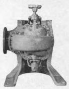
VICTORY SHIP AUX. CIRCULATING PUMP 3000 G.P.M.—10.9 PSI—reconditioned with ABS certificate. Model 12LAS Worthington. Immediate delivery. Vertical motor for this pump—25 HP 230 volts DC—650/875 R.P.M. New impeller available.
