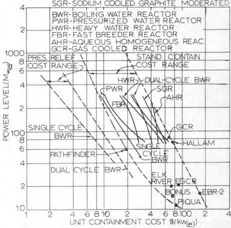
Figure 1-Unit containment cost versus plant size and type of reactor.
