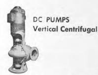
2-WORTHINGTON Circulating Pumps, vertical volute, Type 16"-LAS-2, 5600 GPM, 10 PSI, with G.E. Motors, 20/40 HP, 230 Volts D.C.
