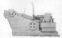
50,000 lb. line pull at 8/10 F.P.M. Declutchable free-wheeling drum-2 outboard gypsies. Mfg. by Jaeger. Levelwind—used with 11/4" wire rope. Drum size 253/4"; between flanges-25"; diameter of flange 50". Driven through torque converter by G.M. 6-71 diesel. Heat exchanger cooled. Can convert to radiator. Used very little. Guaran-
