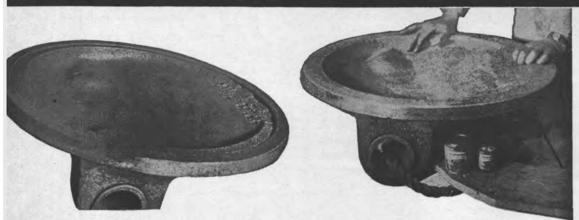
25" clapper valve for a Navy vessel repaired by Cordobond Strong-Back method.
