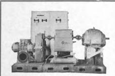
WATEROUS 1406 CARGO PUMPS WITH GYROL DRIVE 1400 GPM @ 100 PSI-268 RPM. Gy-
