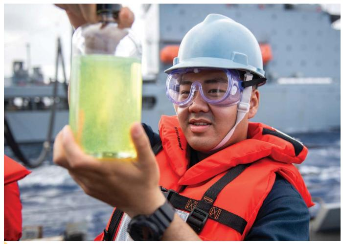
Gas Turbine System Technician (Mechanical) 3rd Class Raymond Htut inspects a fuel sample for color and clarity aboard the Arleigh Burke-class guidedmissile destroyer USS Curtis Wilbur (DDG 54) during a replenishment-at-sea with the fleet replenishment oiler USNS John Ericsson (T-A0 194)
