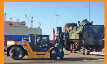
Dual Purpose RoRo; 3.7m Lift With 2.8m Drive Height; 25 Tonne Capacity
