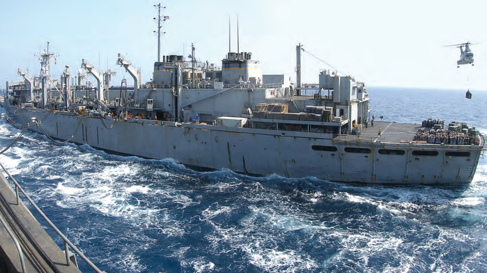
USNS SUPPLY T-AO conducting six CONREP station and simultaneous VERTREP to USS GEORGE WASHINGTON CVN-73 in the Central Arabian Gulf in 2002. (U.S. Navy photo).
