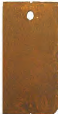
VOS treated steel coupon-270 day corrosion test
