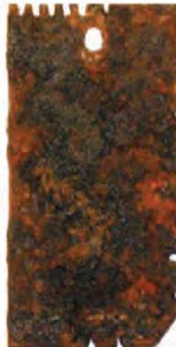
Untreated steel coupon-270 day corrosion test
