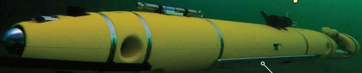
The AUV DeepLeng navigates autonomously in a frozen lake during field tests in Sweden.
