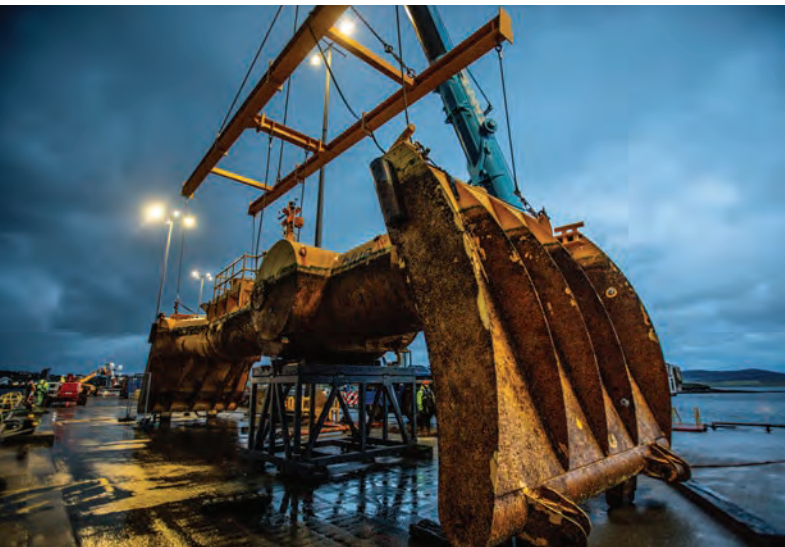
The front of the machine has this big slope plate that ensures that the bow always stays submerged. Waves are over topping (the unit) and that’s a natural load shedding mechanism.
