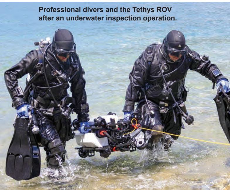
Underwater drone from Tethys Robotics with the DVL500 Compact from Nortek, which facilitates inspection work thanks to reliable positioning.
