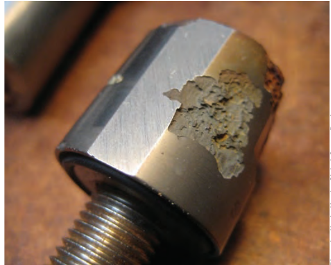
Figure 2 Corrosion of non-DFARS Titanium 6-4. The aluminum rich side corroded due to galvanic action.
