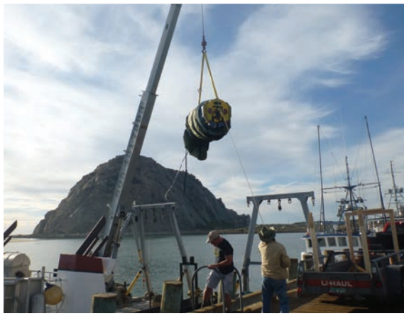
Ample free deck space, low freeboard, an A-frame, and a crane are all requirements for deployment.
