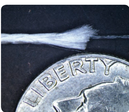
Left A sample of fiber optic fishing line with the inner fiber optic core exposed, next to a United States quarter for scale. The outer diameter of the fishing line is less than one millimeter.
