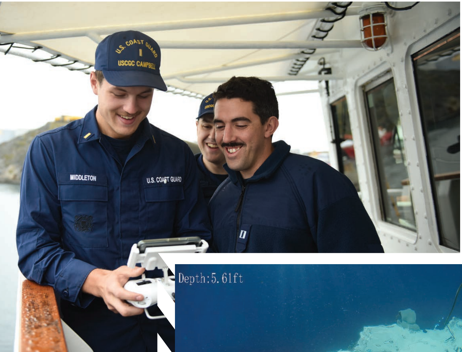
Above: ENS Liam Middleton, LT Stephen Hills and ET1 Douglas Locklear run the FiFish Remotely Operated Vehicle (ROV) to inspect under the waterline of the CGC Campbell. Right: Screen grab from the FiFish Remotely Operated Vehicle (ROV) looking up at the CGC Campbell from below the water line. U.S. Coast Guard photo by SN Kate Kilroy
