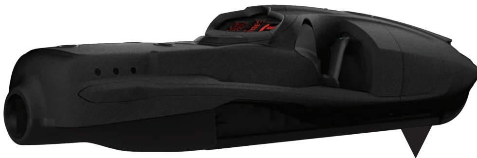
The Rotinor Black Shadow diver delivery system can be used to place detonating charges near mines.
