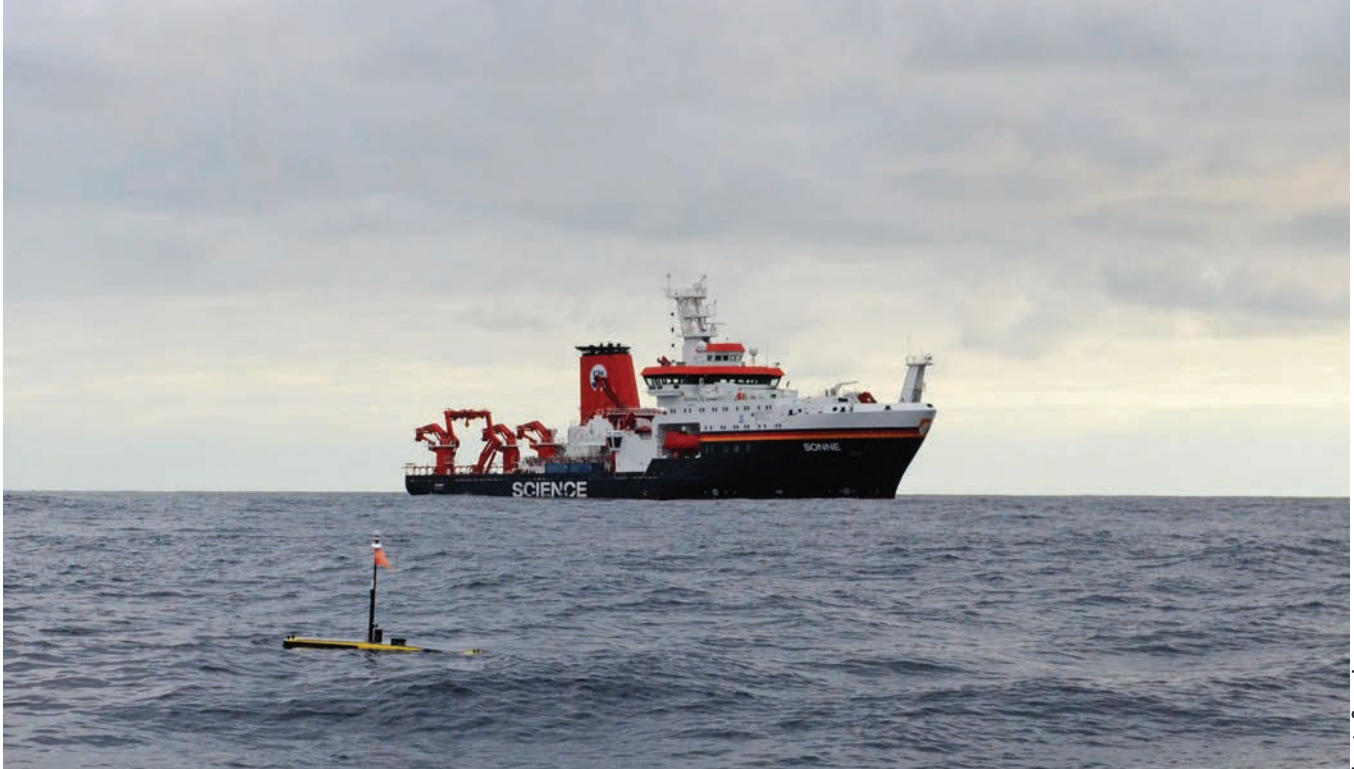
German research vessel Sonne and a Wave Glider unmanned surface vessel (USV) were used to harvest data from AMTs. USVs can now also perform GPS-Acoustic measurements.
