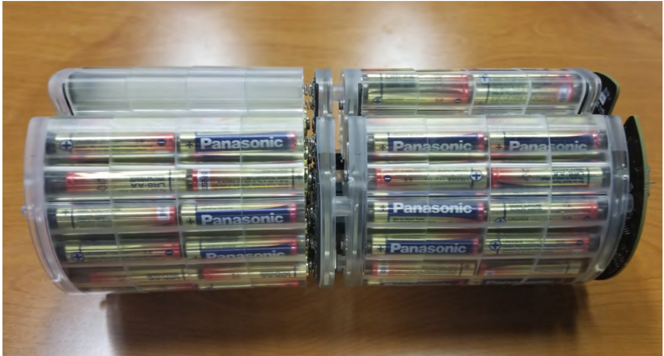
Figure 5: A Typical Alkaline Battery Pack for a Micro-UUV
