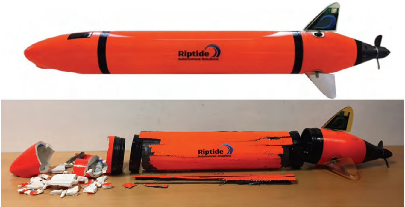
Figure 3. Results of Failure Testing of the Micro-UUV Hull.
