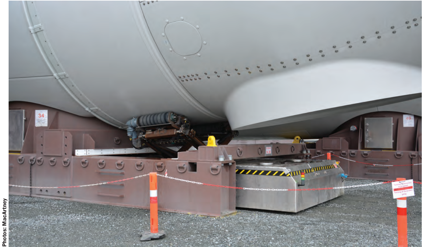
The wind turbine nacelle and hub interface with the generator rotation tool.
