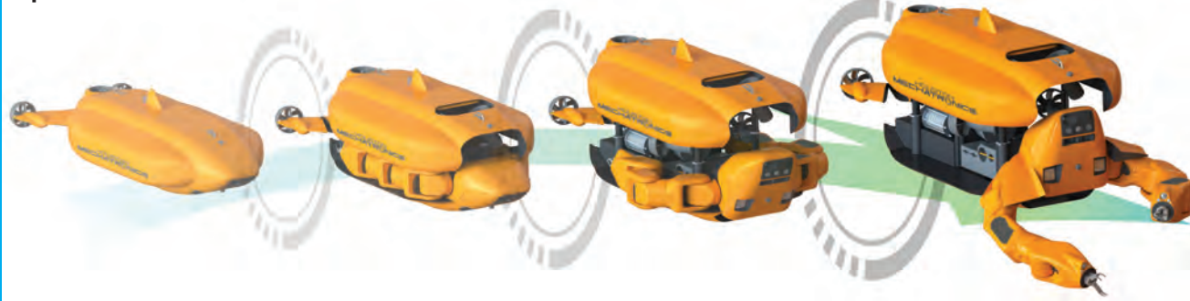
Aquanaut is able to transform from an AUV to an ROV.
