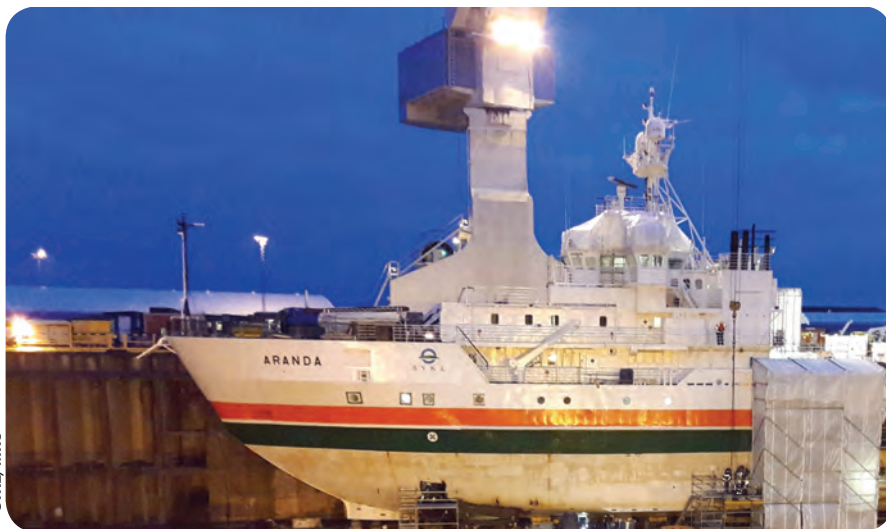
The 59.2m long and 13.8m wide ice-going research vessel Aranda has retained the conventional shafting, while an electrically powered Schottel Pump Jet of type SPJ 132 RD is to be installed as a new auxiliary propulsion unit.
