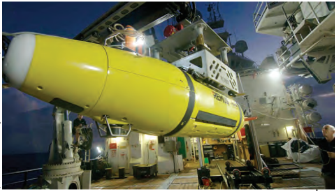
The AUV returns to the R/V Petrel. The autonomous underwater vehicle can operate on a submerged run for up to 20 hours.
