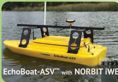
Above: A multibeam survey using EchoBoat-ASV integrated with NORBIT iWBMBc Compact Widebeam Multibeam Sonar with integrated INS/GNSS and real-time sound velocity probe.
