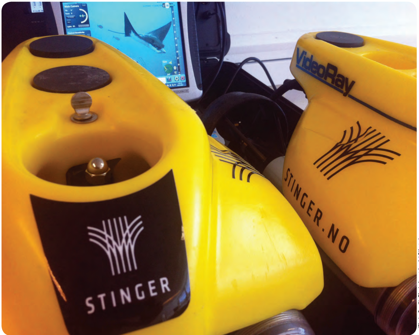
Two of Stinger's VideoRay Pro 4 ROVs.
