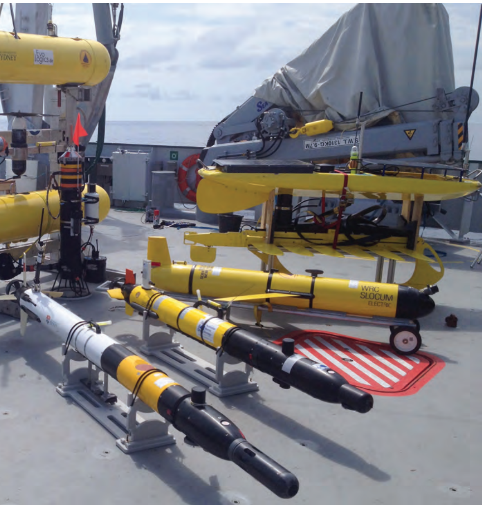
Several classes of autonomous underwater vehicles await deployment on the deck of the Falkor, off the coast of western Australia.
