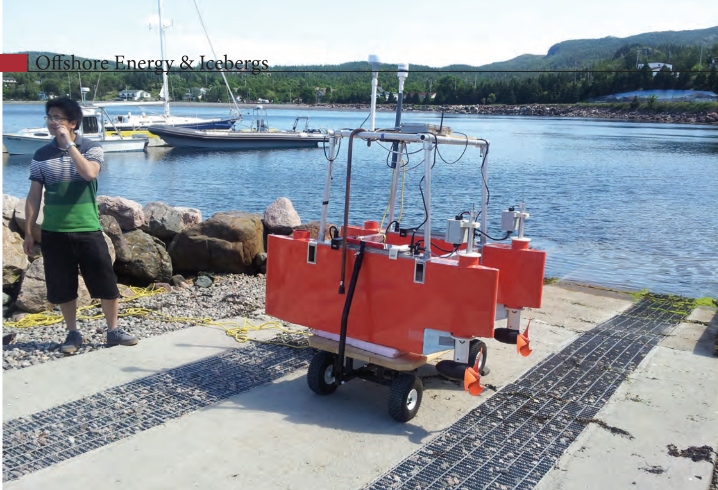
AOSL staff transporting the unmanned "spar shaped" vehicle to a test tank.
