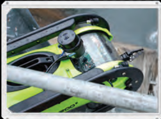
LBV150/200-4 defining portable ROV capability
