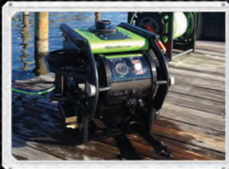
LBV300-5 versatile dual vertical thruster ROV system
