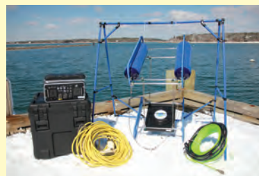
Complete HMS-620 Portable Seismic System (shown with transducer suspended on display frame)
