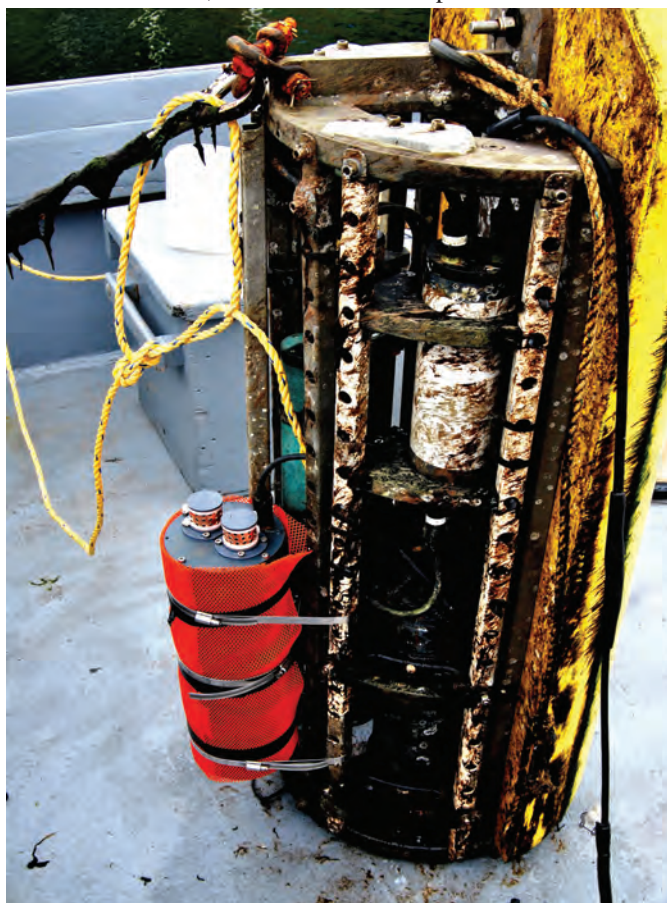
SeaFET with no biofouling after long-term deployment .
