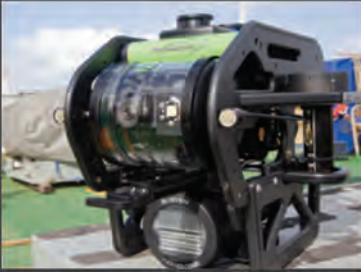
LBV300-5 - versatile dual vertical thruster ROV system.
