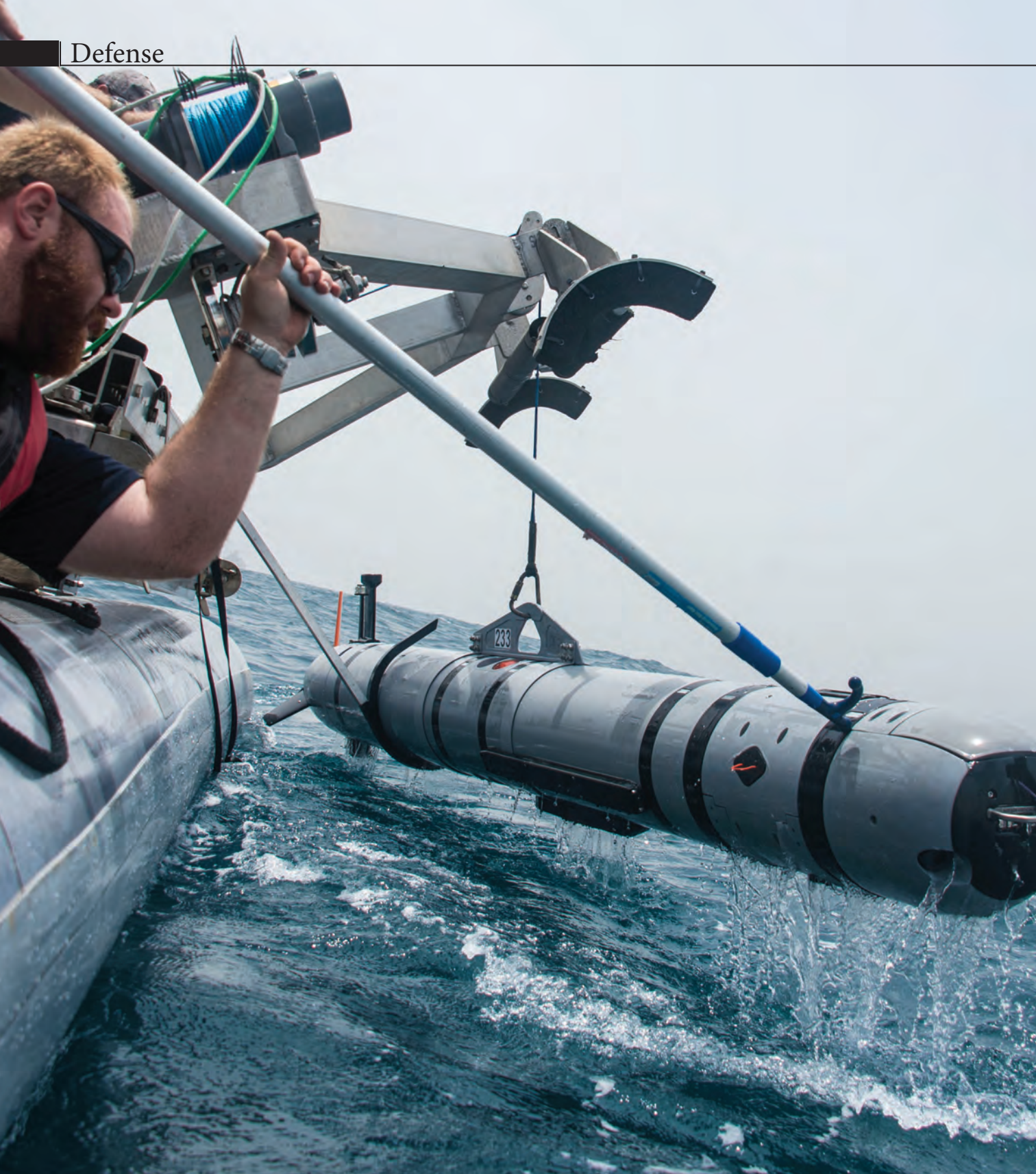
U.S. Navy MK 18 Mod 2 (Hydroid REMUS 600) Vehicle Recovery During Mine Countermeasure Mission.
