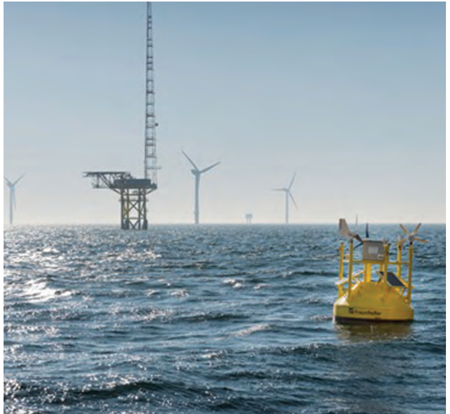
The Fraunhofer IWES' LiDAR wind-measuring buoy was installed near the FINO1 meteorological mast. The buoy measures wind speeds at heights of 40-200 m.
