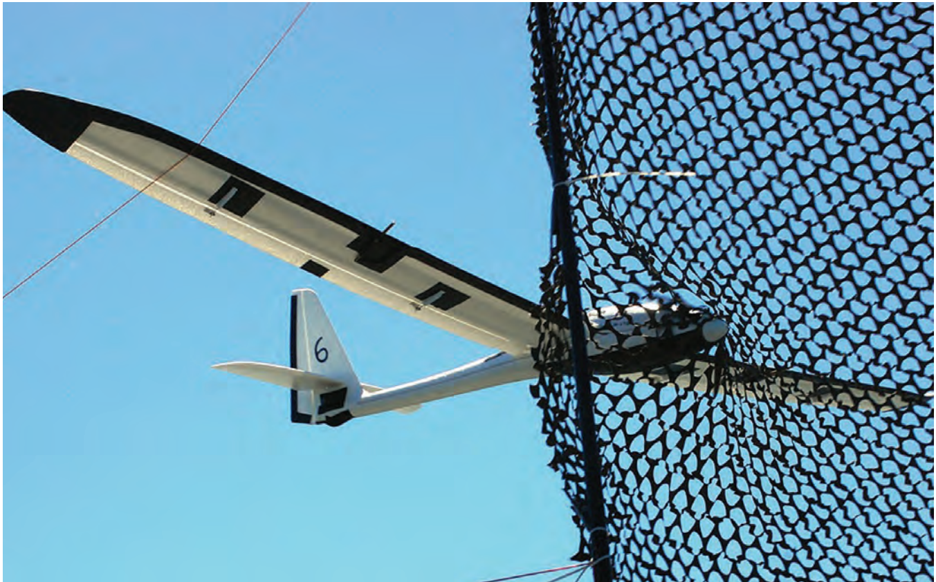
Figure 5 At sea recovery of unmanned aircraft was accomplished by shipboard net capture methods.
