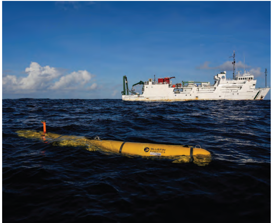
Phoenix International's team onboard the K-O-K research vessel monitor the AUV's position using Ranger 2. The tracking transponder can be seen at the rear of the AUV.
