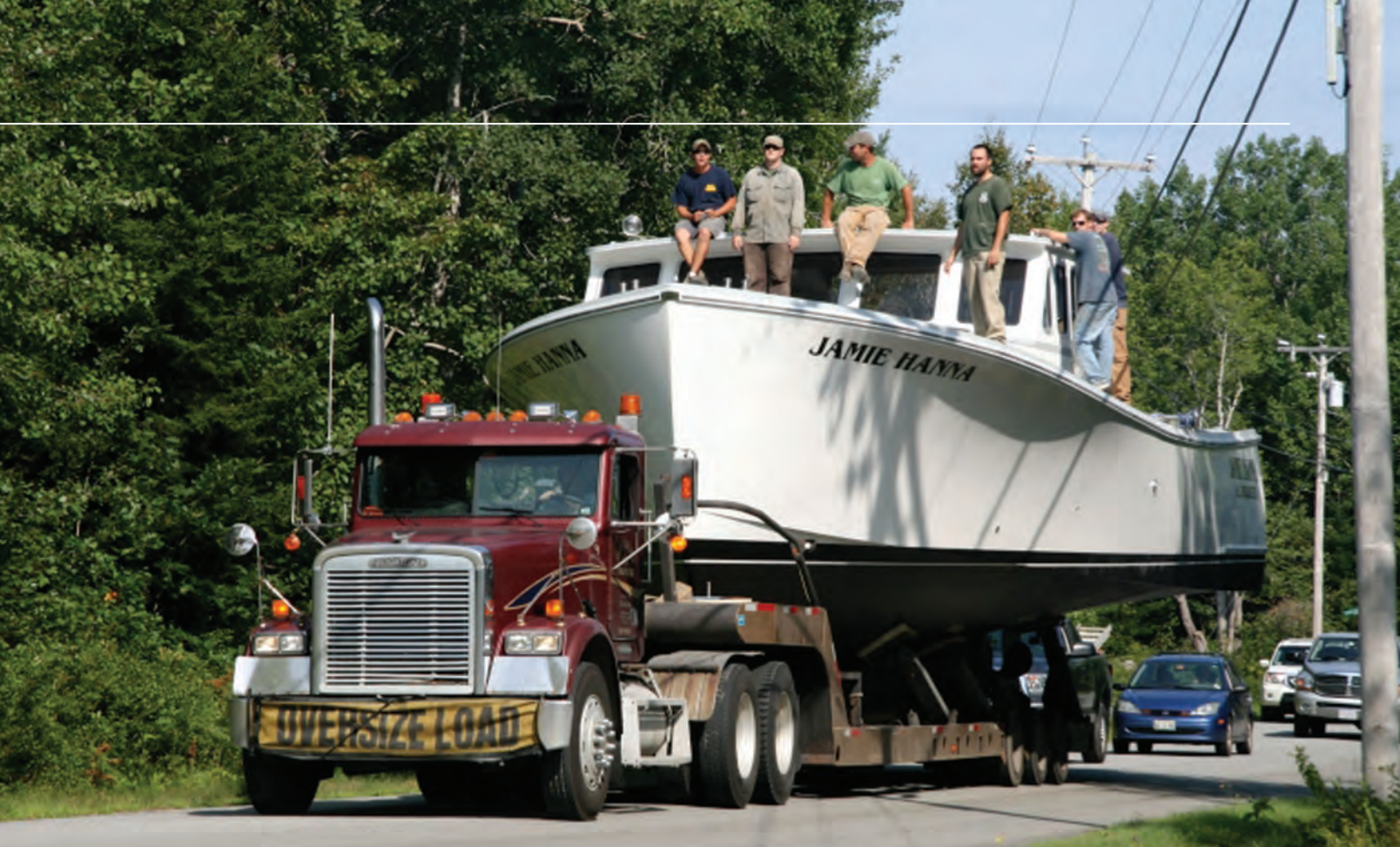
The lead car cleared the road to make way, as the 20 ton hydraulic trailer inched along and a crew on the pilothouse roof lifted phone lines and branches.
