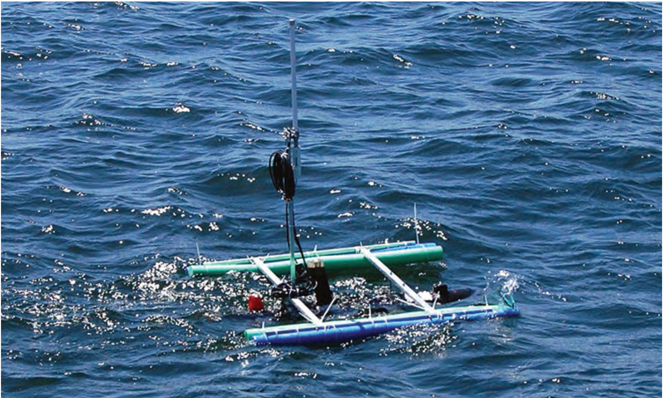
Figure 2 During the REP-12 exercise autonomous underwater vessels (AUVs) (below) from several manufacturers communicated via acoustic modems using DTN communication protocols with each other and with autonomous surface vessels (ASVs) (above).
