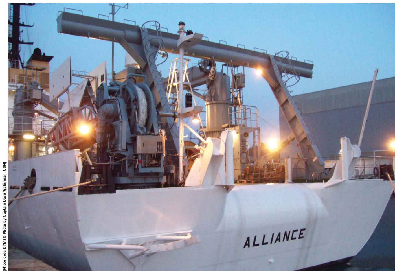
The stern shows the unique capability to tow sophisticated arrays and systems for underwater research.
