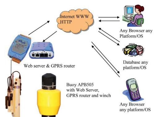
Web server with dynamic HTTP using GRPS router to the WWW: Many users can connect at any time without interrupting measuring sequence at the platform.
