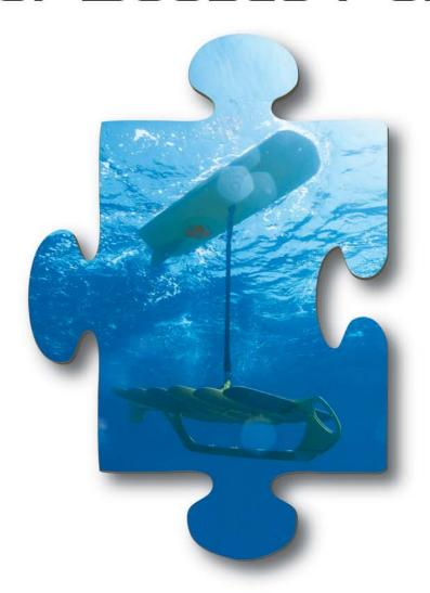
The **Wave Glider** by Liquid Robotics is a versatile platform ready for subsea support. With proven meteorology and oceanography payloads you can monitor ocean conditions in near-real time. The Gateway configuration provides telemetry between fixed and mobile undersea nodes and operators ashore. Using innovative wave energy propulsion, persistent presence in the ocean is now available. Capitalize on this innovation to bring improved operational economics and safety to your operations today.
