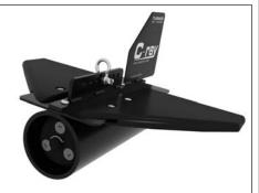
C3 installed in C-ray Deployment Body, part of the C-FINS package.
