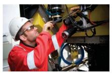
James Rae, S3 ROV Pilot Technician, adjusting the camera pan and tilt unit on an S3 ROV.
