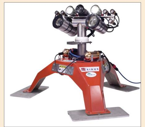
scaling lasers allows for image scaling and object distance measurement.
