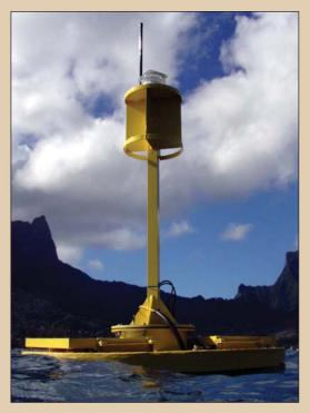
Information gathered from the range of instruments on the mooring needs to be transferred in some way onshore. Typically, data from buoys is relayed to onshore information centres via mobile telephone networks, by radio transfer or by cable. www.macartney.com
