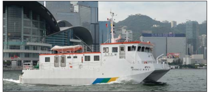
The HKHO survey vessel shown here fitted with dual head EM3000 high resolution multibeam system, which is being upgraded to the EM3002.
