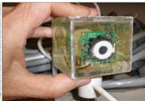
Figure 12.37: Potting Set-Up with Epoxy Potting Compound
