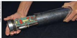
Figure 5.41: Camera with Jam Jar Endcap
