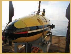
out pre-programmed inspection missions in deep water without physical link to the surface. The deep water trials took place with the local support of ECA's partner in the USA, Harvey Lynch Inc. The vehicle was launched from an Oceaneering vessel hired by BP. Between the 6th and the 15th of July, ALISTAR 3000 executed numerous missions at 4450 ft on a 9" x 13" pipe-in-pipe flowline around BP's King Field.
