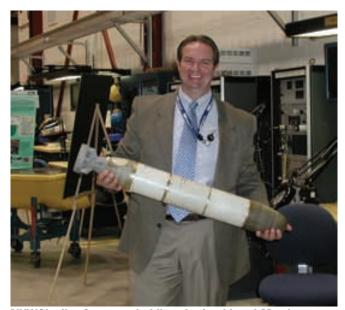
NUWC's Jim Spressor holding the Lockheed Martin EMATT Submarine Target Practice AUV, the smallest of the UUV fleet. (Photo Credit: Maggie L. Merrill, MTR)
