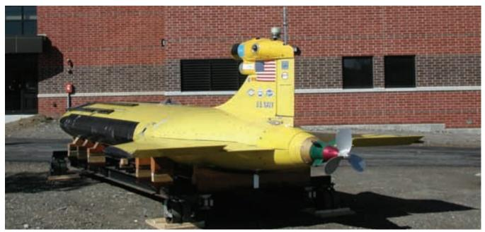
MANTA is a large scale test vehicle which was developed to deal with large payloads and untraditional Concepts of Operations (CONOPS). It is over 34 feet long and displaces nearly 32,000 pounds of water. It can carry up to 5000 pounds of payload and it is modular and reconfigurable to conduct many different types of experiments. (Photo Credit: Maggie L. Merrill, MTR)
