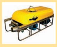
Stingray is capable of easily interfacing with other user-provided devices via multiple RS-232, RS-485, analog, and digital interfaces. The Stingray vehicle has two built-in slide rails, designed for the easy installation of additional buoyancy, tools, cameras, lights, sensors, frames and/ or any other device that the job requires. Stingray comes standard with three optional connectors and one additional camera connector. These standard connectors make future device upgrades simple.
