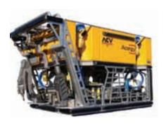
Acergy Core Vehicle (ACV) line, are the product of close collaboration with Acergy, a seabed-to-surface engineering and construction contractor for the offshore oil and gas industry. Schilling was selected by Acergy in 2006 to produce the standard ROV system for the company's next-generation remote intervention fleet. The ACV is based on Schilling's standard
