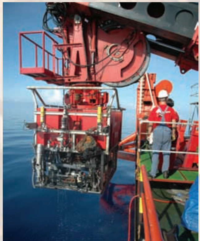
Remote Operated Vehicle recovering to ship with chimney sample. (Photo Credit: Nautilus Minerals)
