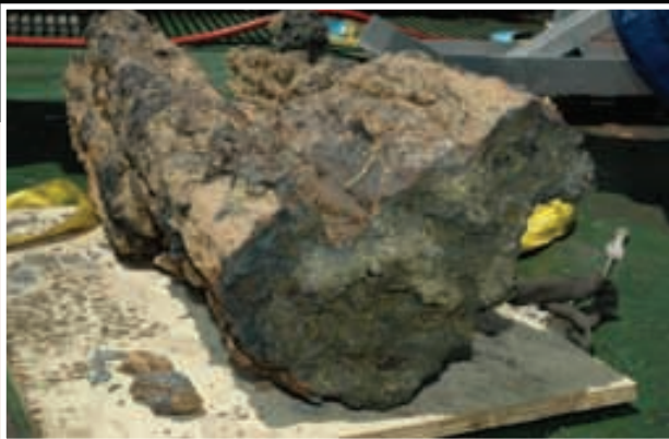
Above: Sample of a Black Smoker on deck being prepared for mineral content analysis. (Photo Credit: Nautilus Minerals)
