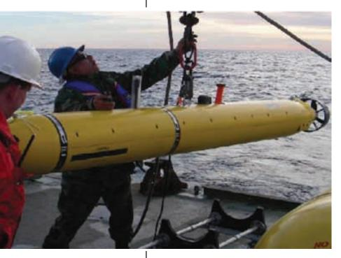
vehicles equipped with QinetiQ's synthetic aperture sonar (SAS) system.
