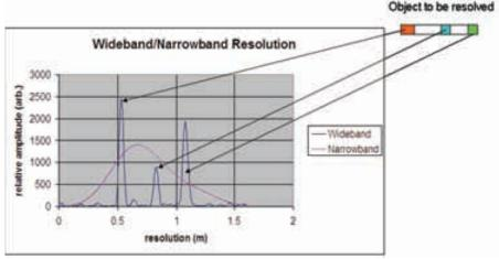
threats where older CW/narrowband Illustration of Resolving Power of Wideband Sonar.
