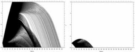
Raytrace for Downward Refracting Sound Speed Profile for Cerberus Vertical Cerberus is designed to work alone Field of View (left hand side) and narrow field of view sonar (right hand side).
