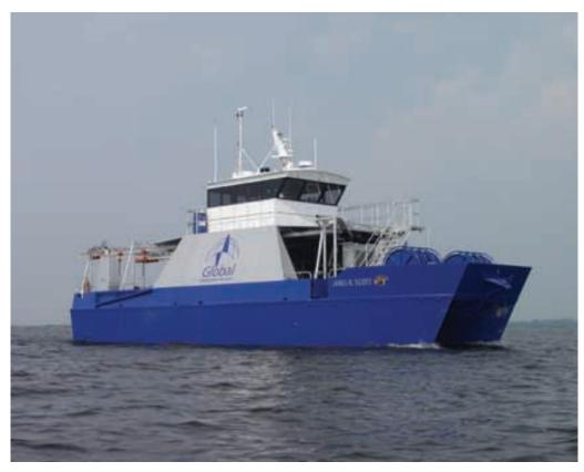
The James H. Scott on sea trials near the builder's shipyard. The catamaran design makes for an inherently stable vessel.
