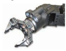
Schilling Robotics' new integrated wrist camera for TITAN manipulators features a titanium camera housing for protection and internal cabling that is designed to eliminate cable snags and abrasions. The high-resolution color camera, which includes LED lights with two illumination levels, can be ordered in either NTSC or PAL format. The depth rating is 4000 m.
