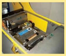
gration of several types of sensors and incorporates all the necessary pipe work and valves while allowing accessibility to the sensors for routine maintenance. Data is logged onboard and then transmitted to shore by GSM phone links and satellite systems.
