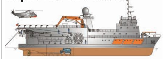
Complete twin-screw medium speed propulsion packages have been ordered from MAN B&W for a twin set of 65 m offshore research vessels. The twins will each be specified and equipped for specific operational tasks, i.e. seismic sourcing and seismic recording. The vessels are designated as an OBC Source Vessel and an OBC (Ocean Bottom Cable) Recorder Vessel, respectively.
