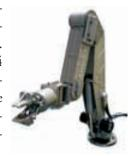
arate enclosure to the manipulator forearm, eliminating the subsea slave controller, slave cable, and 79-pin wiring harness. The new design also reduces Titan system weight by approximately 18 kg (40 lb) in air and 9 kg (20 lb) in water. The standard depth rating has increased to 4,000 m, and a 7,000-m model is also available.
