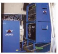
designed for surveys in shallow water, with land/water interface, hazardous areas, and areas requiring rapid environmental assessment. It features area coverage rates as high as 70 sq. km/hr and collects data with a high-accuracy laser, mounted in the aircraft floor.
