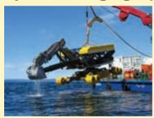
Nexans has developed a terrain dredger/sub-sea intervention system called the Spider. The Spider combines powered tracks with an articulated walking leg system, enabling it to function in uneven sub-sea terrain with up to 35 degrees slope. It is built to work in water depths of approximately 1,000 m. The Spider's movements are controlled by operators located aboard a support vessel, it is launched via a specialized Launch & Recovery System (LARS). Power and signals between the vessel and Spider
