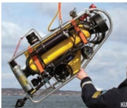
Engineering a contract for two Easytrak Portable subsea tracking systems through its partner CA Clase AB of Göteborg. Easytrak is a USBL tracking system that can provide vital location information on moving targets such as divers and ROVs operating out of sight underwater, and will be primarily used in the authority's search and rescue.
