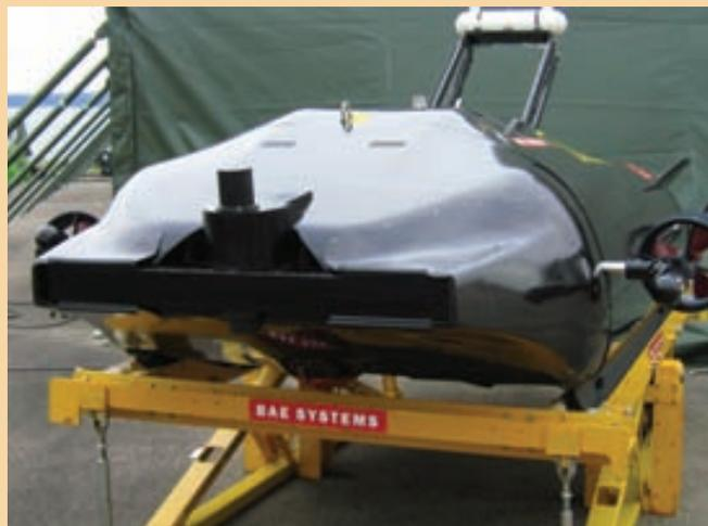
information and receive control commands. It is believed that this was the first time that a Forward Looking MCM sonar has been fitted to an AUV.
