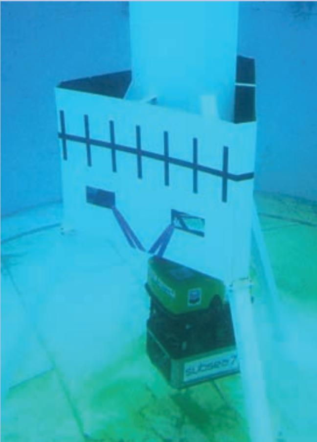
**Prototype Autonomous Underwater Vehicle passing through a structure during tank trials, without tether.**
