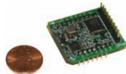
PNI Sensor Corporation announces availability of the MagIC ASIC. When used in conjunction with PNI's SEN-XY magneto-inductive sensors, the MagIC facilitates six times greater magnetic resolution and sample rates than the current PNI solution. The MagIC is a new magneto-inductive drive circuit enabling PNI's SEN-XY to more precisely and rapidly sense magnetic fields while drawing very little power.
