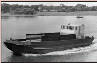
After Luther Blount built his first boat, a 77' steel catamaran, he bid and won a job to construct a fuel oil service vessel using the same catamaran concept based on two cylindrical floats which he dubbed the "twin tube." This design was succeeded by a progression of larger and more complex vessels resulting in a quantum expansion of the shipyard.
