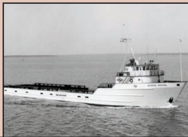
In the 1970s Blount designed and built offshore supply vessels for the U.S. oil industry. The largest of these vessels at 192 feet long were equipped to carry 3,900 cubic feet of drilling mud in six tanks, 350,000 gallons of drill water and had a deck cargo of 640 long tons.
