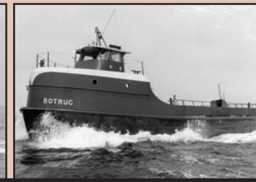
During the late 1950s, Blount designed the Botruc for the offshore oil and gas industry in Southern Louisiana. The Botruc series, as the name implies, bears a strong resemblance to a standard pick-up truck with the cab forward and a cargo space behind the cab.
