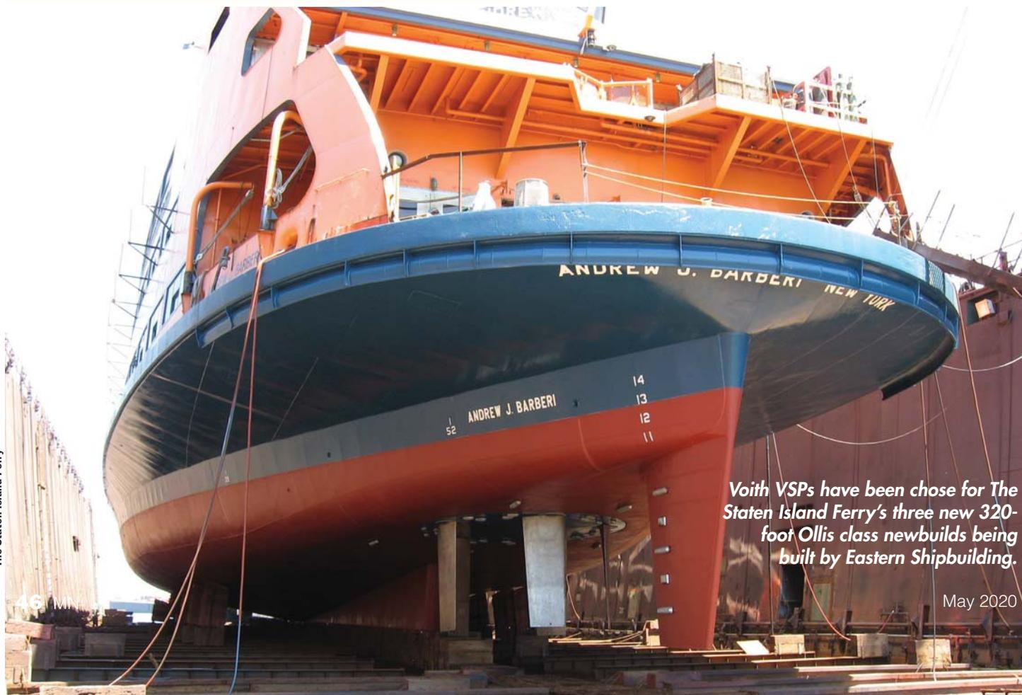
*Voith VSPs have been chosen for The Staten Island Ferry's three new 320-foot Ollis class newbuilds being built by Eastern Shipbuilding.*
